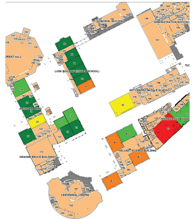
Linking condition findings graphically through a data management tool highlighting low scoring room area condition in a red and orange colour
